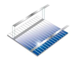
Base-material: ETP Copper foil, soft, double-side tin cladding
